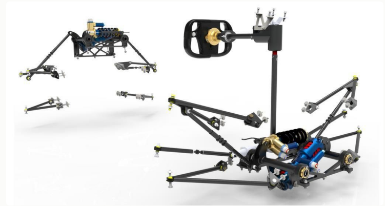
The control arm and tie rod swing on different centres and lengths, so through travel their outer ends want different fore and aft positions. The difference comes out as steer.
